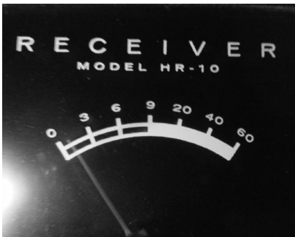
Figure 17.2 — A Heathkit HR-10 S meter, with a full scale deflection of 60 dB over S-9. Vintage receivers can have quite accurate S meters, providing they are calibrated at the frequency of operation. Modern receivers tend to have much more uniform response throughout the HF spectrum.
