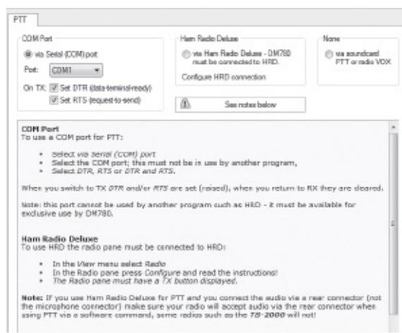
**Figure 1.5 – In this configuration screen from *Ham Radio Deluxe* you’ll notice that COM 1 has been selected as the transmit/receive keying port.**
