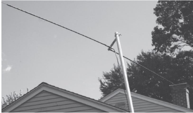
**Figure 4.3 – A 20-meter dipole made from two Hamstick-style mobile antennas joined together.**
