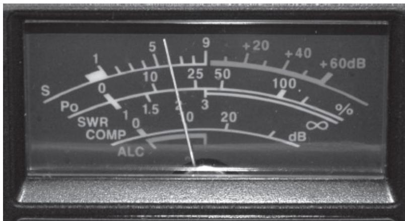
In this ICOM transceiver meter, the ALC “safe zone” is indicated with a red bracket at the bottom. As long as the needle stays within the zone, you have a decent chance of transmitting a clean signal.
