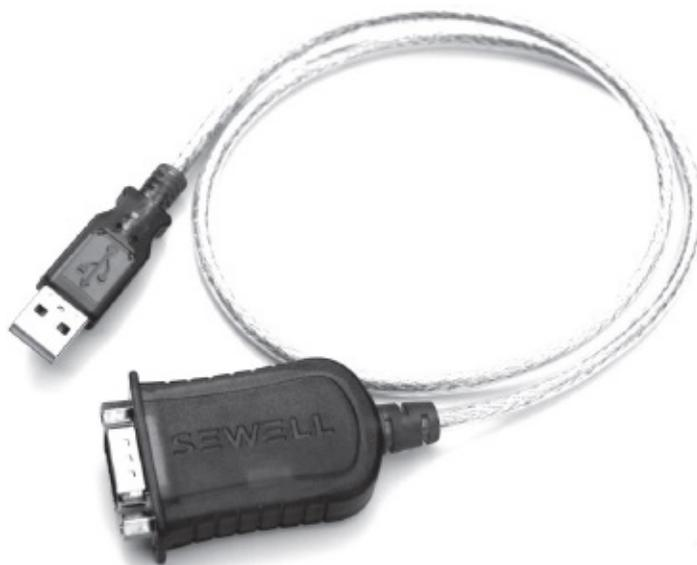
A USB-to-serial adapter cable like this one makes it possible to attach serial interfaces to computers that only have USB ports.
