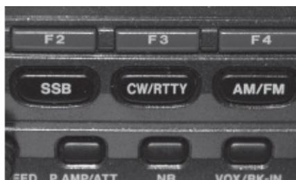
The CW/RTTY mode button on an ICOM transceiver. But is it AFSK RTTY (and other digital modes), or FSK RTTY alone? Time to consult the user manual!
